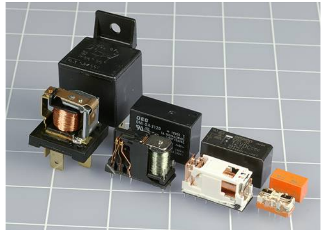
Figure 2-61 A variety of 12-volt relays. See text for details.
