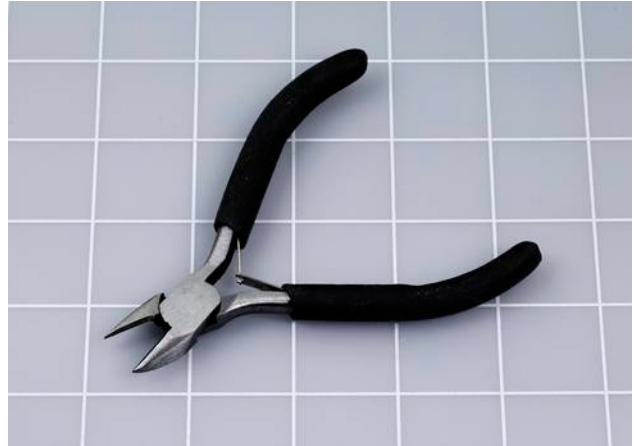
Figure 2-4 Wire cutters should be no more than 5" long.
