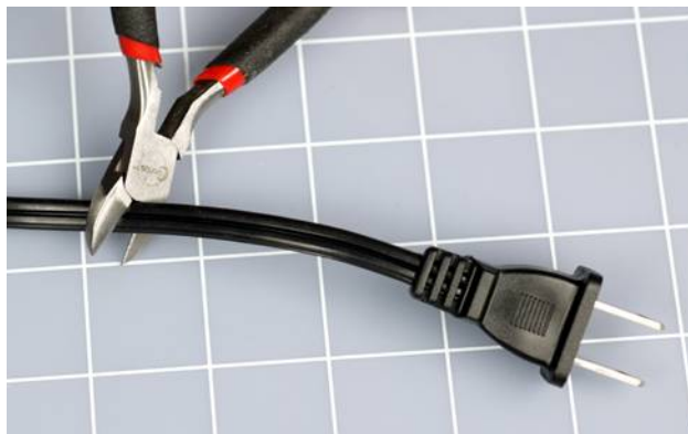
Figure 3-49 Step 1 of 12, to shorten a power cord.
