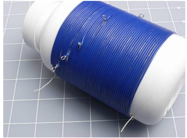
Figure 5-68 The completed coil, wrapped tightly around the bottle.
