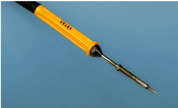
Figure 3-3 A low-wattage soldering iron designed for precise electronics work.
