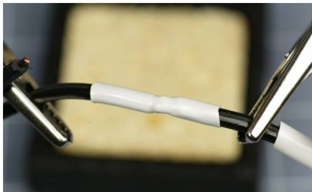
Figure 3-58 Step 10 of 12, to shorten a power cord.
