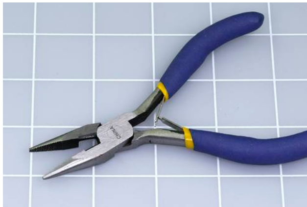
Figure 2-2 Appropriate pliers for electronics work should be no more than 5" long.
