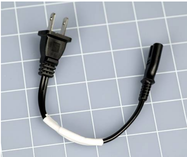
Figure 3-61 The power cord, shortened.
