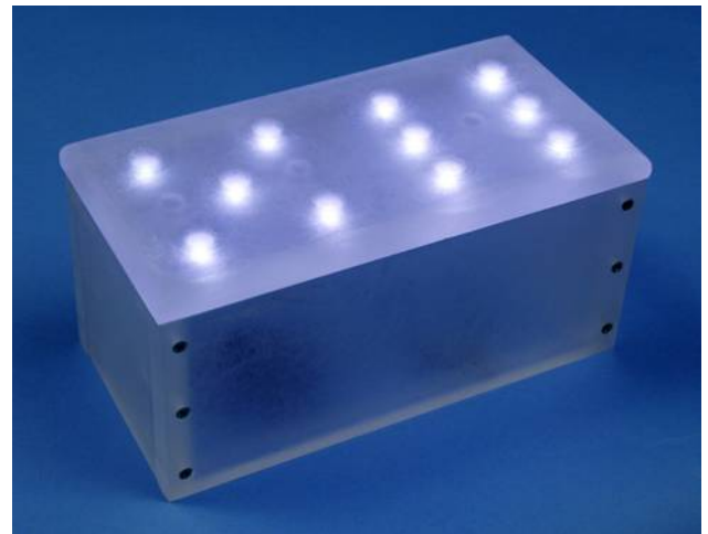
Figure 4-156 This electronic dice display uses 10mm LEDs embedded in a box of sanded polycarbonate plastic.
