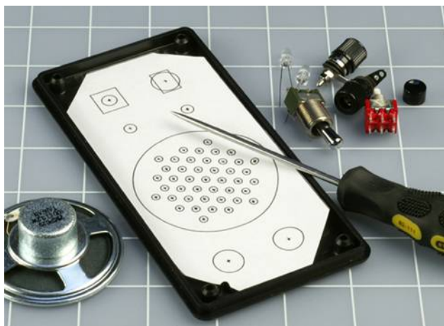
Figure 4-55 A printed layout for the switches, LEDs, and other components has been taped to the underside of the lid of the project box. An awl is pressed through the paper to mark the center of each hole to be drilled in the lid.
