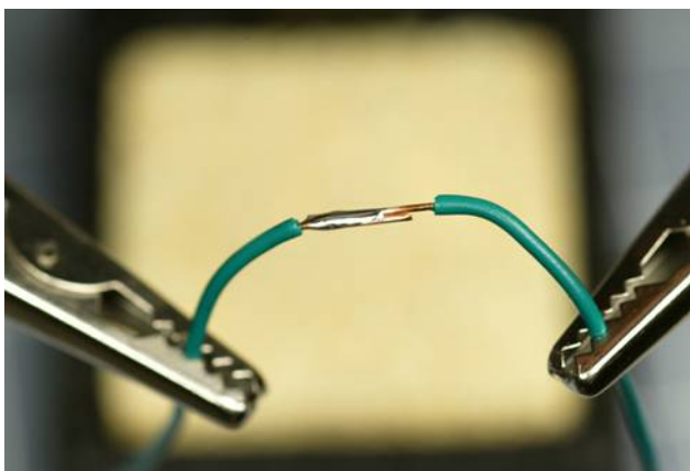
Figure 3-38 The finished joint is shiny, and the solder has spread across the copper wires.
