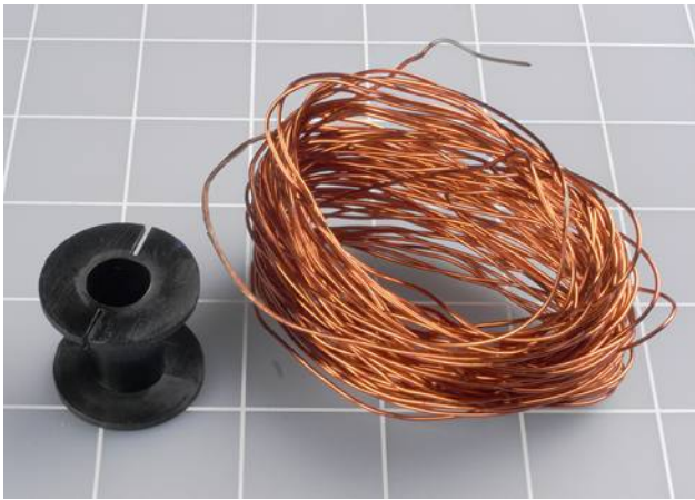
Figure 5-56 The audio crossover coil consists of a plastic spool and some wire. Nothing more.
