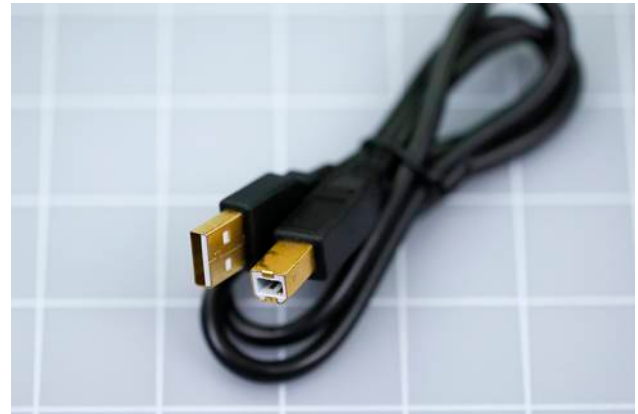
Figure 5-81 You will need this type of USB cable to attach your Arduino board to a USB port on your computer.
