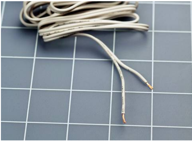
Figure 3-46 The stripped wires.
