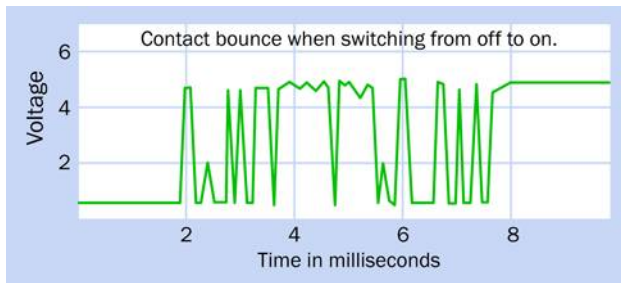
Figure 4-127 Fluctuations created by vibrating contacts when a switch is closed. (Derived from a datasheet at Maxim Integrated corporation.)
