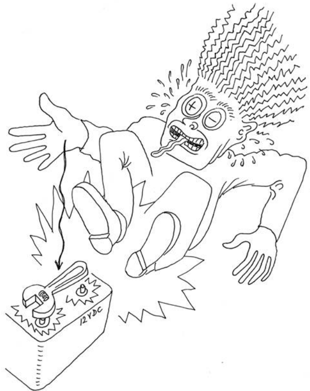
Figure 1-28 Dropping a wrench between the terminals of a car battery will be bad for your health. Short circuits can be dramatic, even at a "mere" 12 volts, if the battery is big enough.
