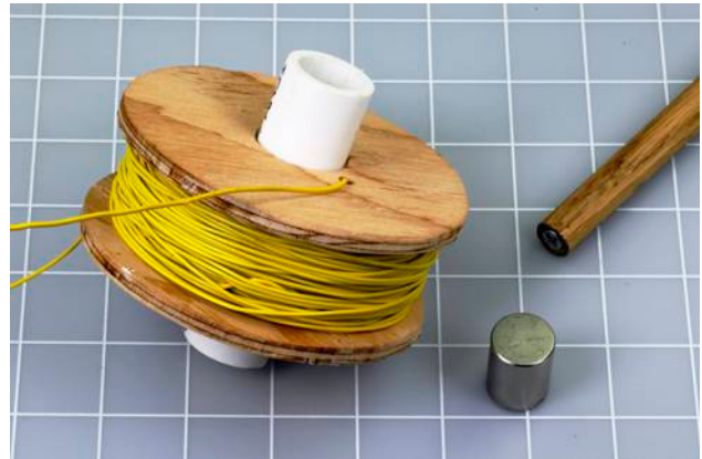
Figure 5-18 Two hundred turns of 22-gauge wire on a home-made spool, with a magnet that attaches itself to a screw in a wooden dowel.
