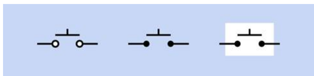
Figure 2-46 Three variants of the pushbutton symbol. The white rectangle is added in this book for clarity, but is not used elsewhere.
