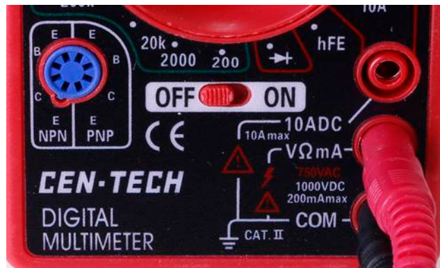
Figure 1-19 Socket functions are split up differently on this meter.
