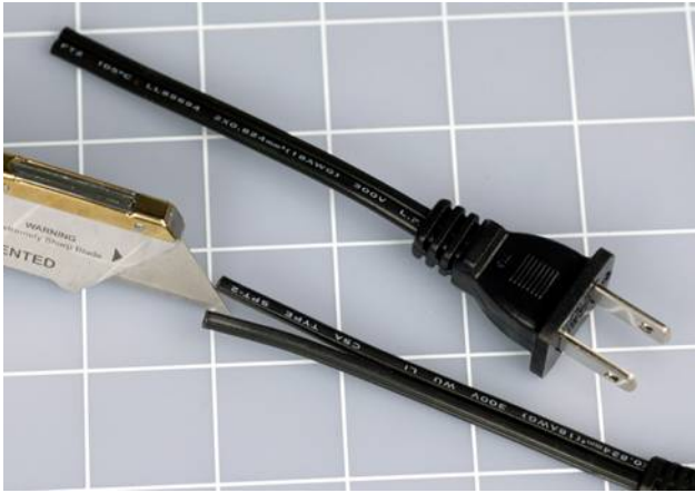
Figure 3-51 Step 3 of 12, to shorten a power cord.
