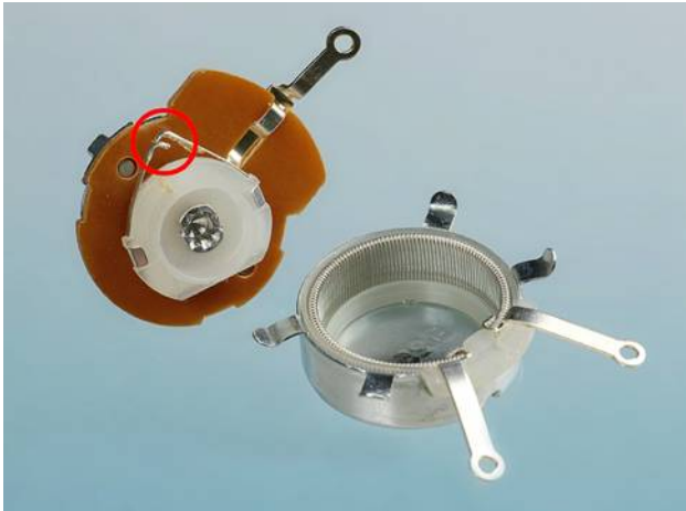
Figure 1-50 The wiper of the potentiometer is circled.
