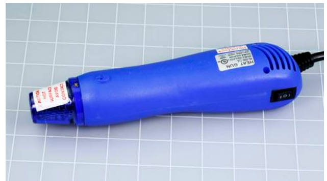
Figure 3-11 A miniature heat gun is slightly easier to handle than the full-sized type.
