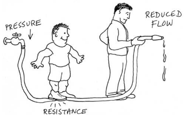
Figure 1-32 Resistance blocks pressure and reduces flow—in water, and in electricity.
