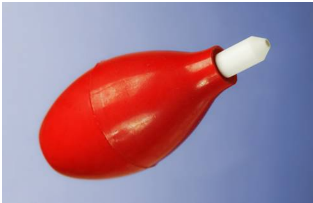
Figure 3-12 To remove a solder joint, you can suck melted solder into this squeezable rubber bulb.
