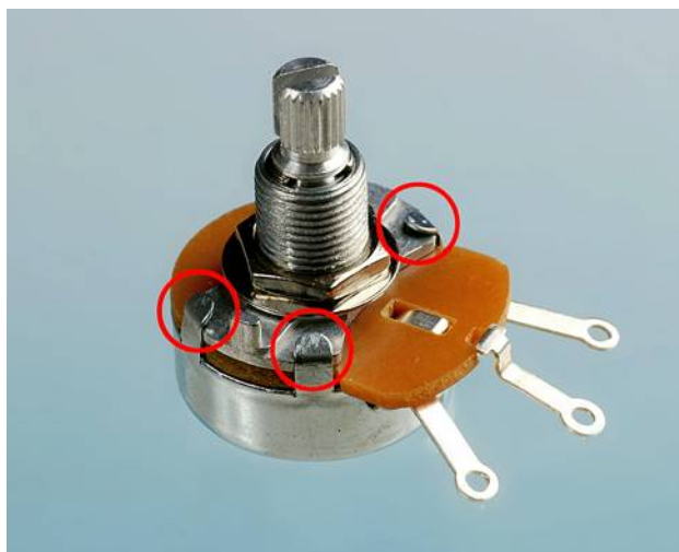
Figure 1-48 The tabs that hold a potentiometer together.
