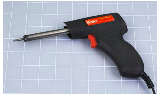
Figure 3-4 A Weller Therma-Boost 30W soldering iron can be useful when working with heavier wire and larger components.
