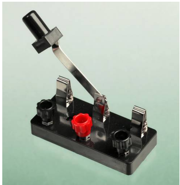
Figure 2-29 A single-pole, double-throw (SPDT) switch connects one pole with a choice of contacts.
