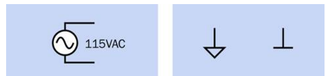
Figure 2-43 Symbolic representation of AC power (left) and chassis in an AC device (right).
