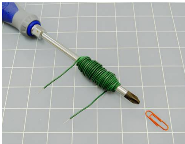
Figure 5-9 This most basic electromagnet is just strong enough to attract a paper clip.
