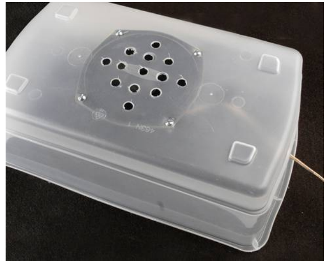
Figure 5-41 A resonant enclosure is necessary if you want to hear some bass (lower frequencies) from your speaker. A cheap plastic storage bin is sufficient for demo purposes.
