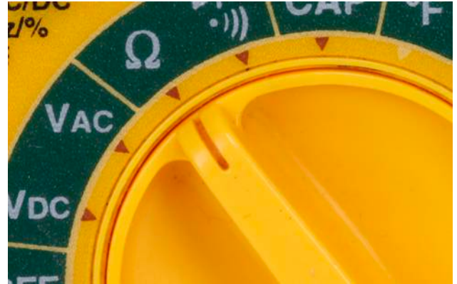
Figure 1-22 On an autoranging meter, just turn the dial to the ohm (omega) symbol.
