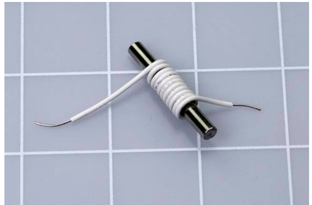
Figure 5-16 Just ten turns of wire can be sufficient to create a small electrical potential when a magnet moves through them.
