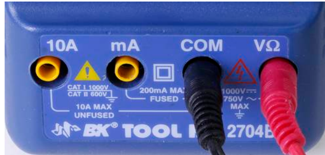
Figure 1-18 Note the labeling of sockets on this meter.
