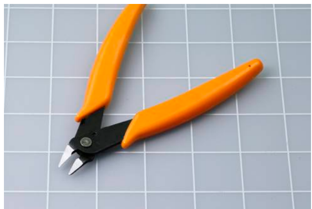
Figure 2-5 Flush cutters can get into smaller spaces than wire cutters.
