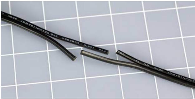
Figure 3-52 Step 4 of 12, to shorten a power cord.
