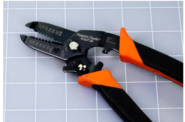
Figure 2-8 The recommended wire strippers are designed for 20-gauge to 30-gauge wire.
