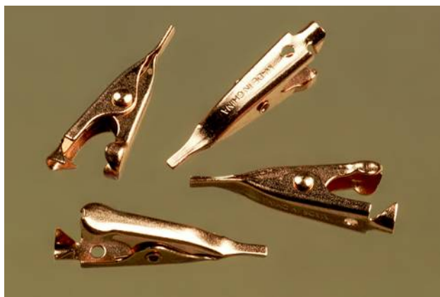
Figure 3-20 These small copper clips absorb heat to protect components when you're soldering them.
