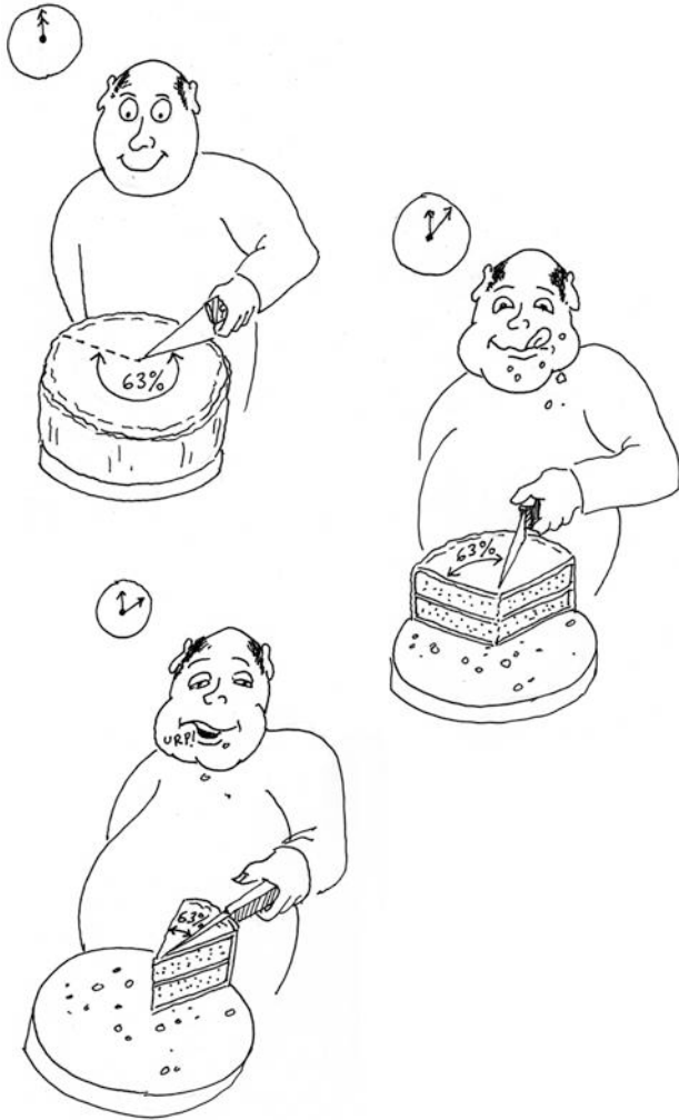
Figure 2-82 If our gourmet always eats just 63% of the cake still on the plate, he “charges up” his stomach in the same way that a capacitor charges itself. No matter how long he keeps at it, the cake is never quite gone and his stomach is never completely filled.
