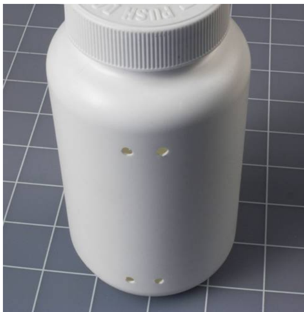
Figure 5-64 The holes will anchor wire wrapped around the bottle.
