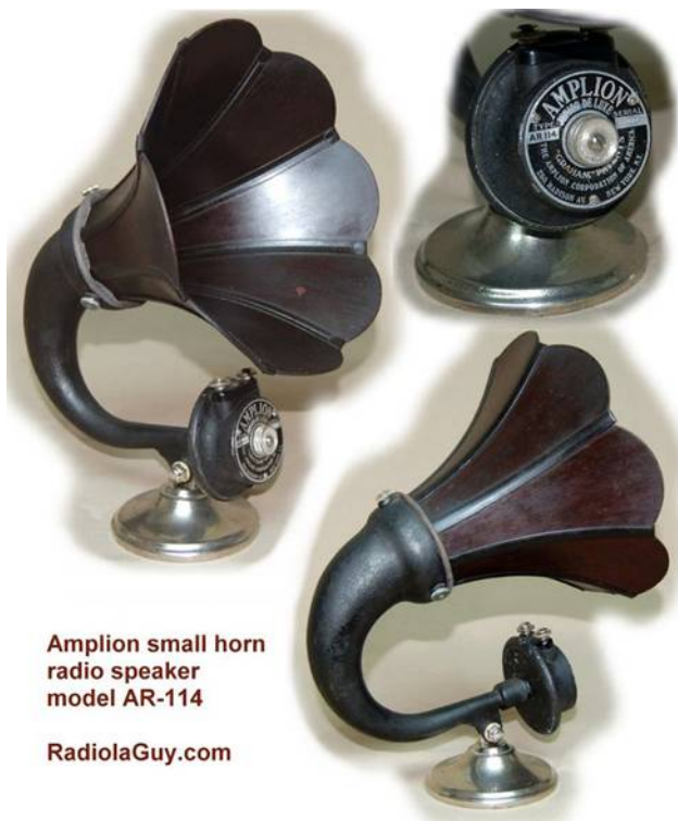
Figure 5-29 This beautiful Amplion AR-114x illustrates the efforts of early designers to maximize efficiency in an era when the power of audio amplifiers was very limited. Photos by “Sonny, the RadiolaGuy.” Many early speakers are illustrated at http://www.radiolaguy.com . Some are for sale.
