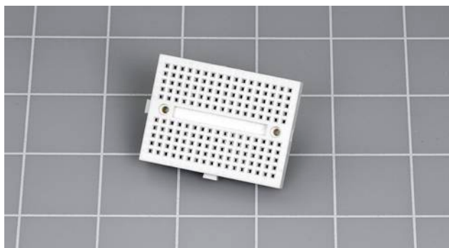
Figure 2-9 A mini-board is not big enough for many of the projects in this book.
