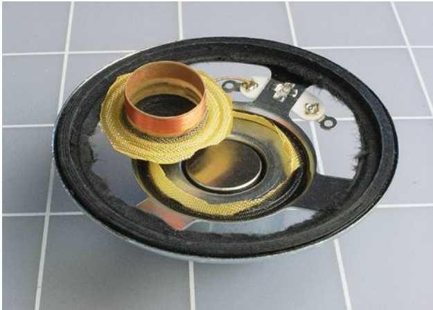
Figure 5-28 The copper coil is normally hidden inside the groove of the magnet, below.
