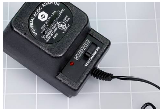
Figure 3-1 This AC adapter plugs into the wall and allows you a choice of DC voltages by moving a small switch.
