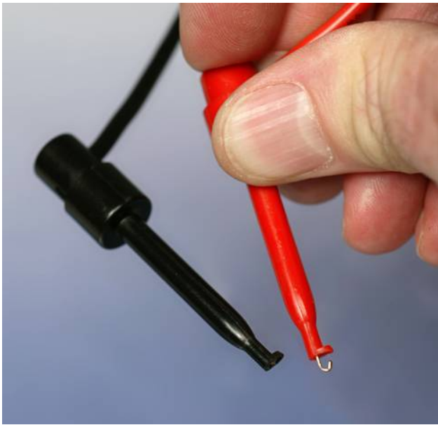
Figure 3-8 These “minigrabbers” on meter leads will grip wires or component leads.
