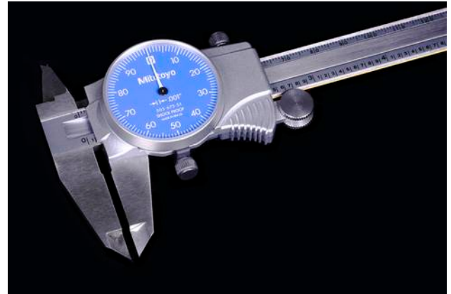
Figure 3-17 Calipers can measure internal and external diameters.
