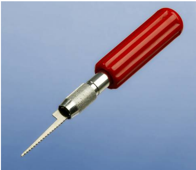
Figure 3-15 Useful for cutting small holes to mount components in plastic boxes.
