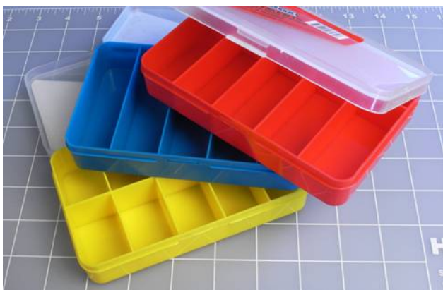
Figure 5-4 Darice Mini-Storage boxes are ideal for components such as resistors, capacitors, and semiconductors. The boxes can be stacked stably, stored on shelves, or grouped in larger boxes. The brand sticker is easily removed after being warmed with a heat gun.
