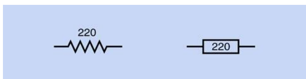
Figure 2-44 Symbol for a resistor in the United States (left) and Europe (right).
